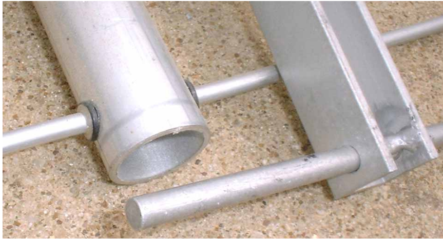
Insulated element mounting on the left, direct on the right.
