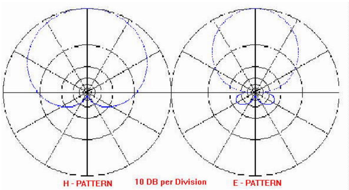
**How does the tape measure beam "measure up?"**
