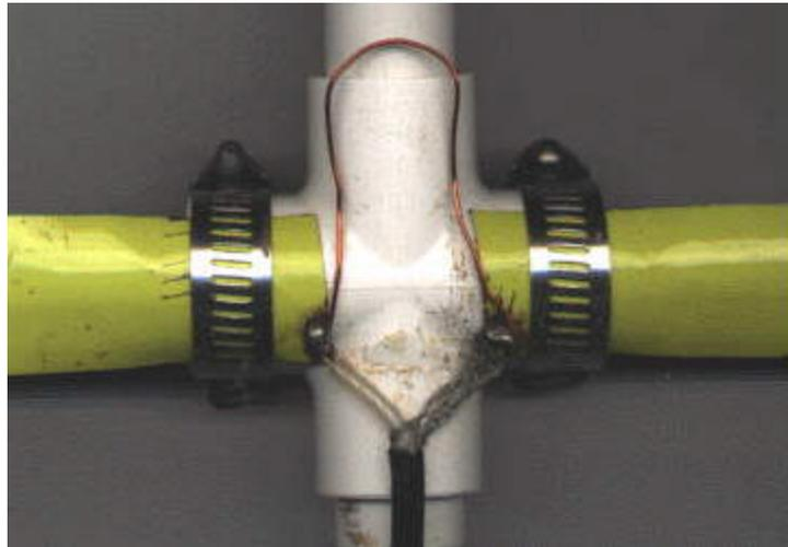
that the SWR was 1:1 at 146.565 Mhz (our Fox-Hunt frequency) when the two elements were spaced approximately 1 inch apart. Figure 1 shows the method used to attach the driven element to the PVC cross.
