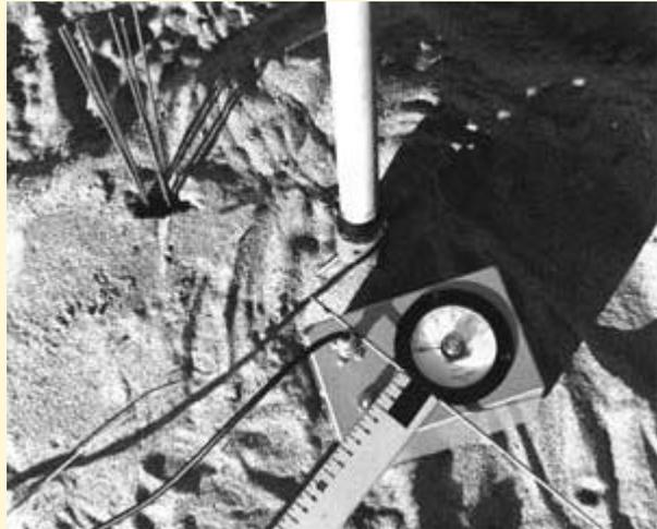
Once the experimenter has confidence in the integrity of the antenna range, it's quite possible to dispense with the receiver and VU meter and use a signal source plus a field strength meter such as the one shown in the photo at right (which also shows an assortment of elements of varying lengths, including one mounted on a meter stick for use in antenna design work).
